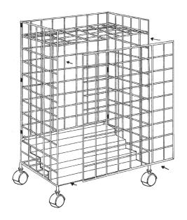
4. Attach front grid (D) to side grids (A). Using small clips, attach grid (C) to grids (A).
